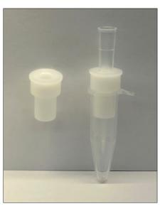
A Peptide Desalting C18 StageTip Adaptor can be inserted into a 1.5 mL microcentrifuge tube (not provided). A Peptide Desalting C18 StageTip #45943 can then be placed through the central hole of the adaptor, such that solutions can pass through StageTip by centrifugation and collect in the bottom of the microcentrifuge tube.
