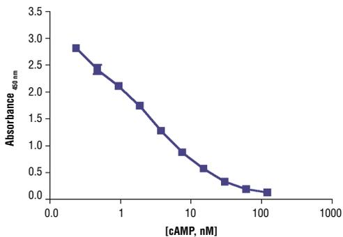
Figure 1: cAMP Standard was diluted in 1X Cell Lysis Buffer #9803 and samples were assayed following the Cyclic AMP XP<sup>®</sup> Assay Kit protocol. This standard curve is for demonstration purposes only; users should generate a standard curve for each sample set in order to accurately determine cAMP concentration.
